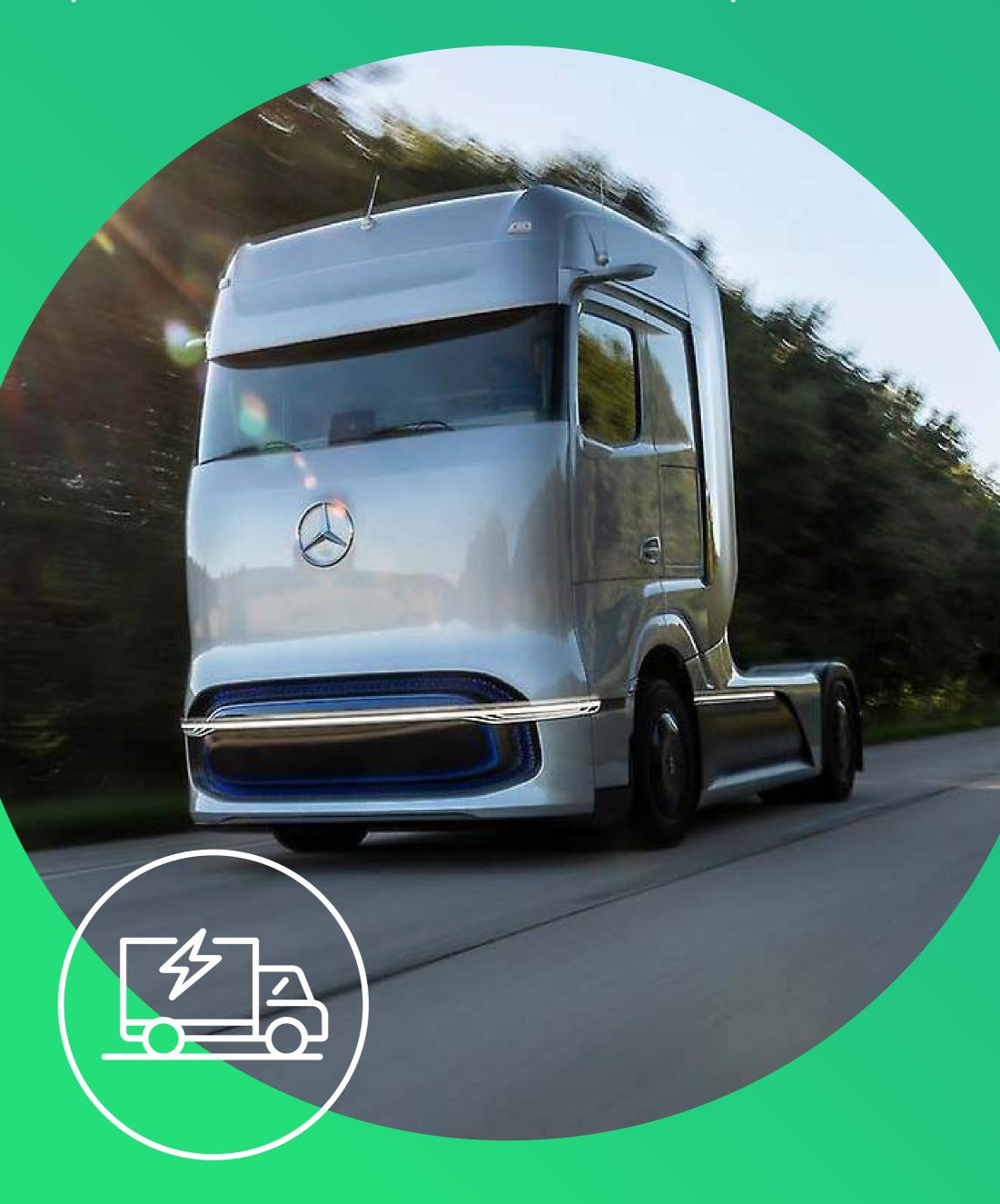
In September 2020, Daimler presented a hydrogen fuel cell concept truck called the Mercedes-Benz GenH2 Truck.
